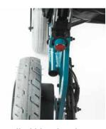
**Overall width reduced** The frames allow for the motors to sit inside and reduce the width.
