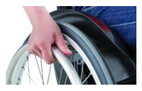
Stainless steel, brushed Less susceptible to scratches, provides good grip Additional weight per wheel: + 400g
