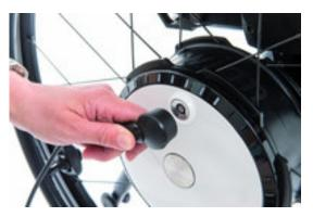
A new feature is the patented EasyConnex charging plug. Using magnetic force, it automatically finds the correct plug-in position.
