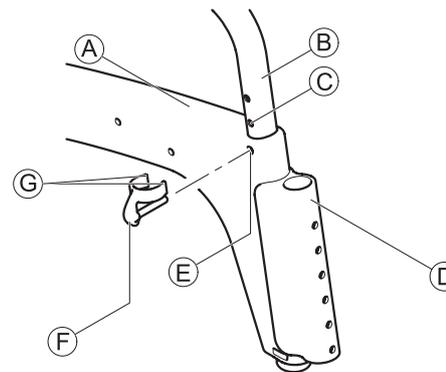
1. Remove the enclosed clips (F) from the bag.
