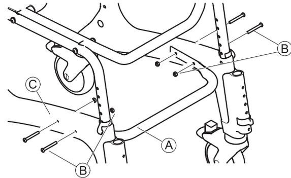
1. Fit the base stabilization tube (A) using the screws and nuts (B) supplied between the side parts (C).
