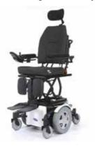
Seat lifter The 300mm seat lifter provides easy access to higher obstacles.
