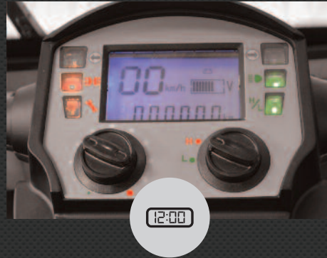
Digital dashboard display Speed, distance travelled and temperature at a glance
