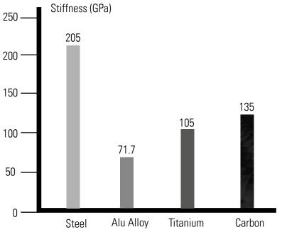
Carbon Fibre Vs Traditional Materials Fibre Excluding steel, which is too heavy, composite Carbon Fibre is stiffer than aluminium and titanium.
