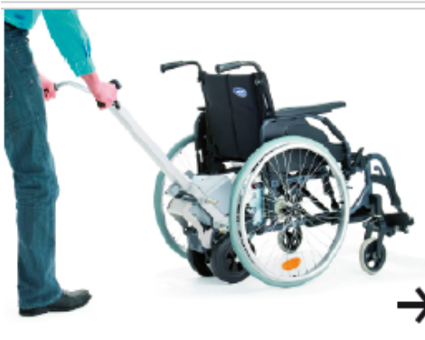
Drive viamobil eco into the bracket ...
